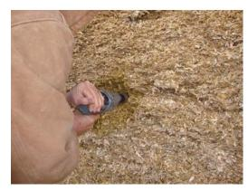
The coring drill is a standard size so by knowing the depth of the hole and weight of the silage removed from the hole, density can be calculated using a spreadsheet
